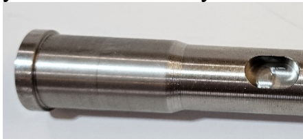
Stem has machined cut out for fork lock
